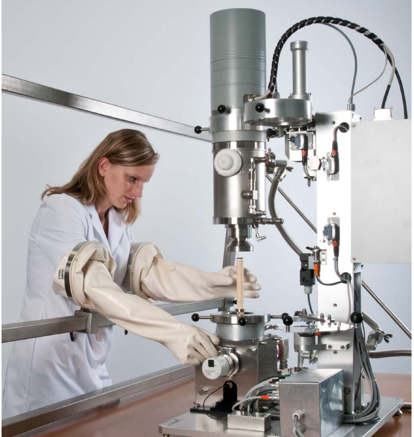
LFA 427 in a mockup glove box
