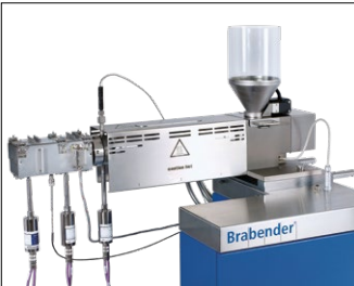
Measuring extruder / Extrusiograph 19/25, Application: Thermoplastics
