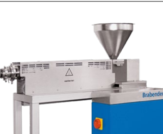
Measuring extruder 30/25 Application: Thermoplastics
