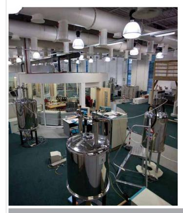
Millburn House has thirteen superconducting magnets for performing NMR, ranging from 850 MHz (proton Larmor frequency) to 100 MHz for solid-state NMR, 700 and 600 MHz for solutionstate NMR and a three magnet solid-state DNP system.
