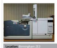
An orthogonal acceleration time-of-flight mass spectrometer with high resolution for the selectivity needed to separate analyte spectra from isobaric interferences and background chemical noise. Identifies the elemental compositions of small molecules.
