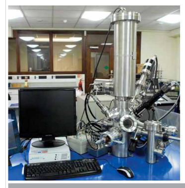
Time-of-flight secondary ion mass spectrometer (TOF-SIMS) instrument for characterisation of surfaces, detection of all elements as well as identification of organic species and thin film profiling.
