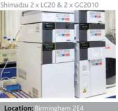
Two HPLC and two GC systems for analysis of molecular materials and nanomaterials.
