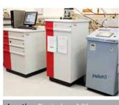
Magnetic Property Measurement System (MPMS) magnetometer utilises Superconducting Quantum Interference Device (SQUID) technology. The MPMS provides solutions for a unique class of sensitive magnetic measurements in key areas such as high-temperature superconductivity, biochemistry, and magnetic recording media.
