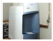
High-performance, matrix-assisted laser desorption/ionisation time-of-flight mass spectrometer featuring parallel position sensitive detection (PSD) technology for confirming protein identification and determining posttranslational modifications.
