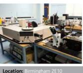
Modular instrument for measuring fluorescence and phosphorescence decays on molecular nanomaterials
