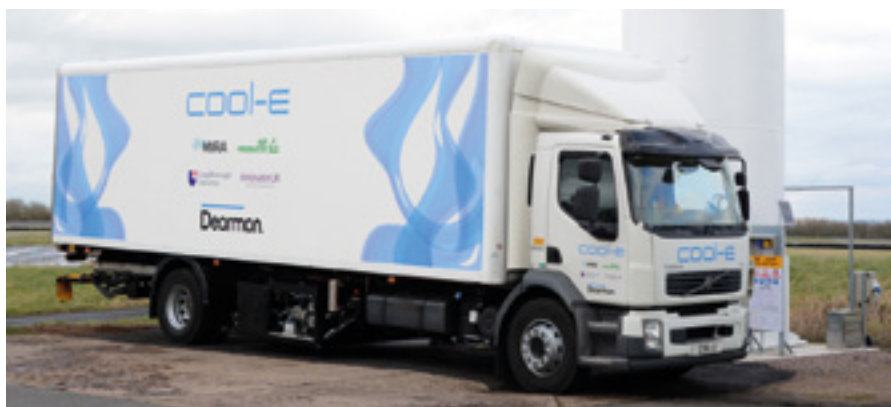
A lorry with a liquid air powered Dearman TRU providing cooling.
